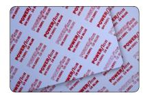
POWER®flon 10 BLUE is a structured PTFE - Gasket - Sheet manufactured by a unique process which provides a high level of fibrillation to overcome the creep relaxation and cold flow problems associated with normal (skived or moulded) PTFE sheets. POWER®flon 10 BLUE is produced from virgin PTFE resin filled with hollow glass micro spheres.
